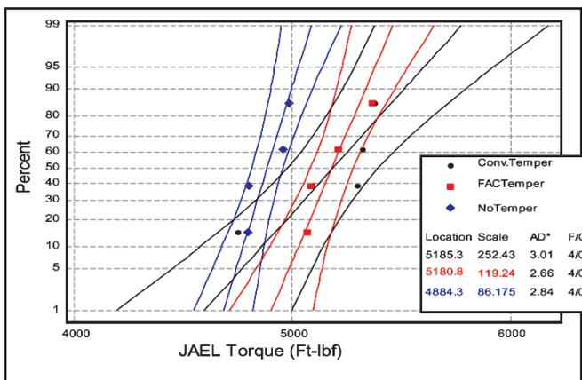
Fig. 7 — Normal probability plot of JAEL strength for various as-quenched and tempering conditions
