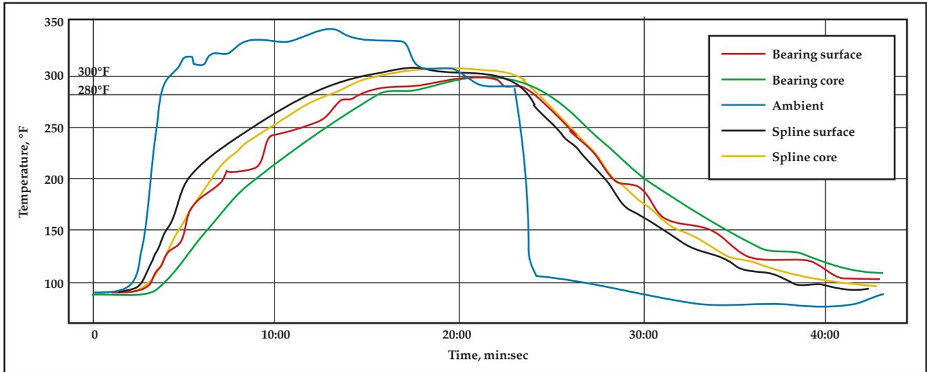
Fig. 3 — Thermal profile by processing time and location on axle shaft for vertical FACT furnace
