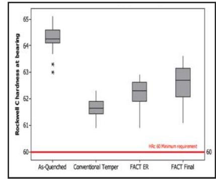
Fig. 4 — Box and whisker plots of HRC at the bearing journal for as quenched, conventional temper, and FACT tempering during equipment run off (ER) and final prove out
