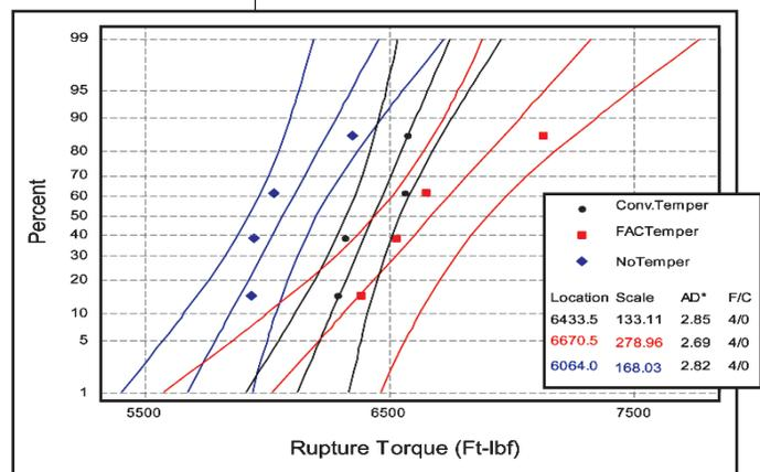
Fig. 8 — Normal probability plot of rupture strength for as-quenched and conventional and FACT treatments
