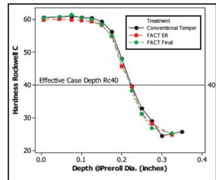
Fig. 5 — Microindentation hardness profiles at the spline cross section for conventional and FACT (equipment run off) samples
