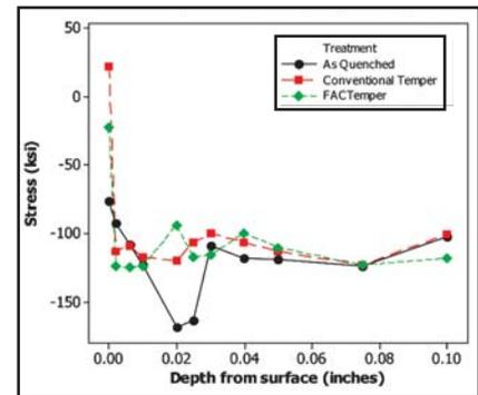
Fig. 6 — Scatter plot of residual stresses as a function of depth from the surface for as-quenched and tempered methods.
