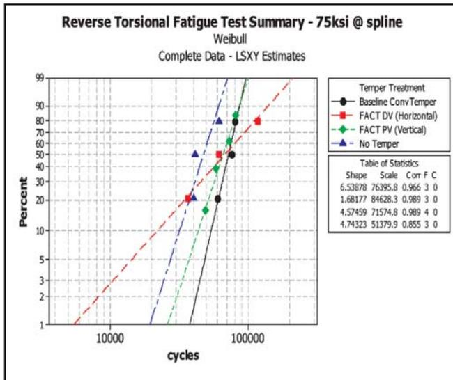
Fig. 9 — Weibull plot of reverse torsional fatigue for various tempering treatments
