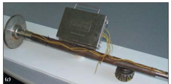
Fig. 1 — Thermocouples located at the spline end (a) and bearing region (b) of the axle shaft and overview of instrumented shaft with data recorder attached (c)
