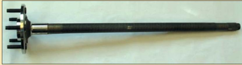
Automotive axle shafts transmit torque from the drive train to the rear wheels, support the vehicle load, and function as the inner race for the wheel bearings. Four key design features of an axle shaft are:
