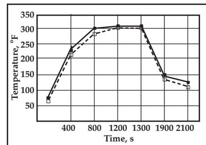
Fig. 2 — Temperature uniformity and repeatability for horizontal FACT furnace. Solid black = mean temperature +1 sigma, hollow square = mean temperature -1 sigma
