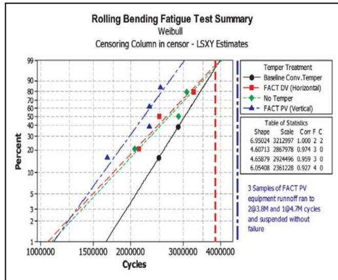
Fig. 10 — Weibull plot of rolling bending fatigue life by tempering treatment
